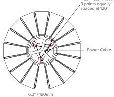
PCD = 6.3" / 160mm .3 points equally spaced at 120°
